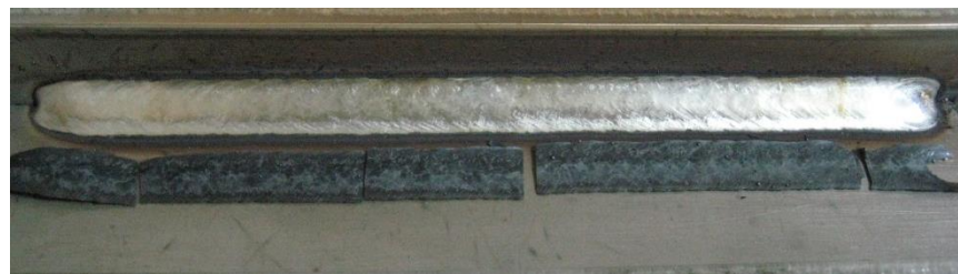
KFW-308L 1.2 mm 200A 32V CO 2 Position: 2F
